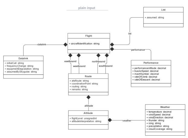
Figure 2. Plain input concept UML diagram
