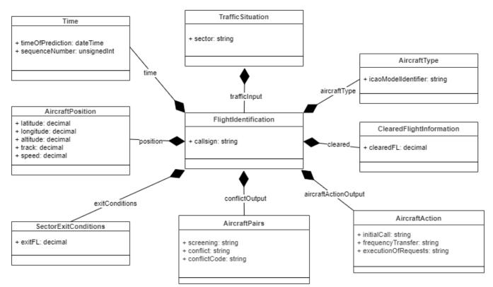
Figure 4. Complexity estimation module UML diagram
